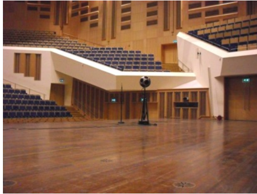
Figure 3.7: In-situ measurement setup on a concert hall stage with a source-receiver distance of 1 m.
