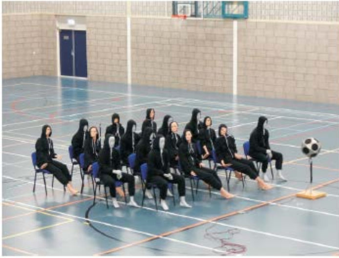
Figure 4.6. The attenuation of direct sound through a group of humans and a group of mannequins has been measured in a sports hall for validation. The picture shows the setup with the group of mannequins.
