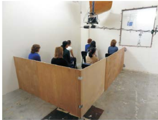
Figure 4.4. Sound absorption measurement setup in the reverberation room with 1 m 2 per chair occupied by 8 women.
